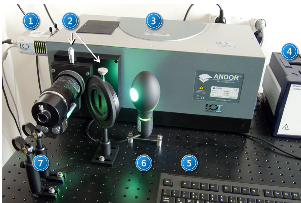
Picture 1. View of apparatus for recording linear emission spectra: 1 – CCD camera; 2 – slits; 3 – spectrometer; 4 – mercury lamp power supply; 5 – computer; 6 – mercury lamp; 7 – mirrors.
